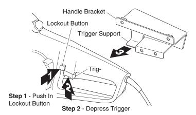
Figure 1 - Attaching Handle Bracket to Chain Saw Handle
